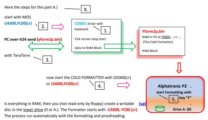
There are only two short messages. **ok - then you win**, otherwise **Error** - is what the disc or the device is not in order. **Repeate!** Then **any more new disks are formatted**. These hard reset key and restart with the MOS at **U5000,FC00** (cr) or **G5000** (cr). (up)
